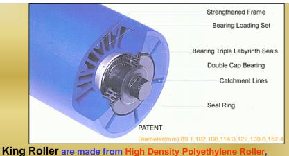
King Roller are made from High Density Polyethylene Roller, the versatility of this material enables us to satisfy a varied range of uses where other plastic and steel roller have failed. The injection molding processes also ensure the high quality and accurate concentricity necessary to carry our brand name.
