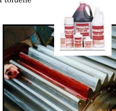
Dykem Steel Red for dynamic contact tooth flank checking
