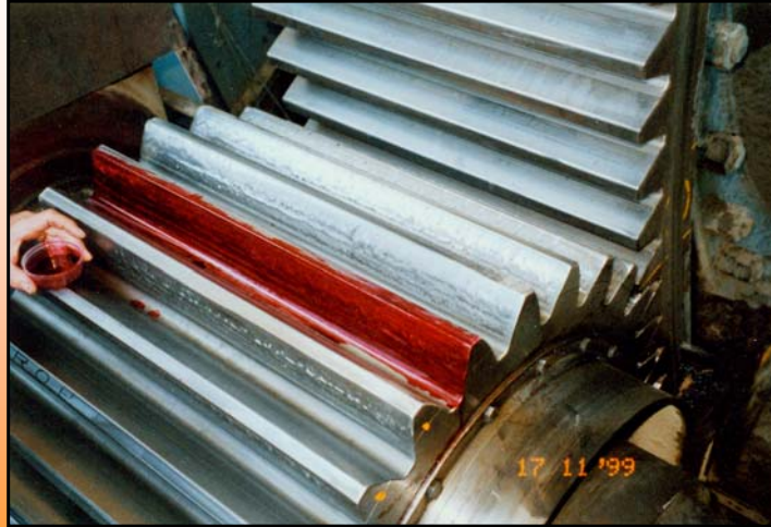
Application of oil resistant colour paint(DYKEM STEEL RED)
