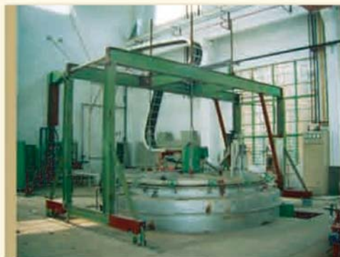
2.0 × 2.8m渗碳炉 2.0 × 2.8m carburizing furnace
