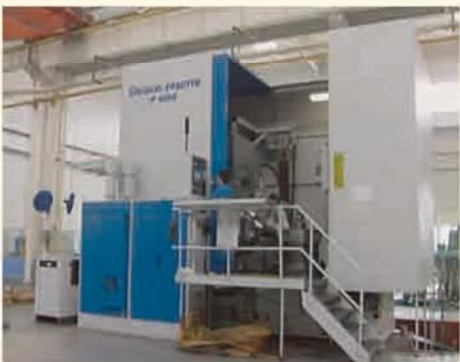
德国普法特高效数控滚齿机 High efficiency CNC hobbing machine from Gleason-Pfauter, Germany
