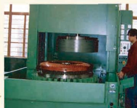
淬火压床 ▶ Quenching press
