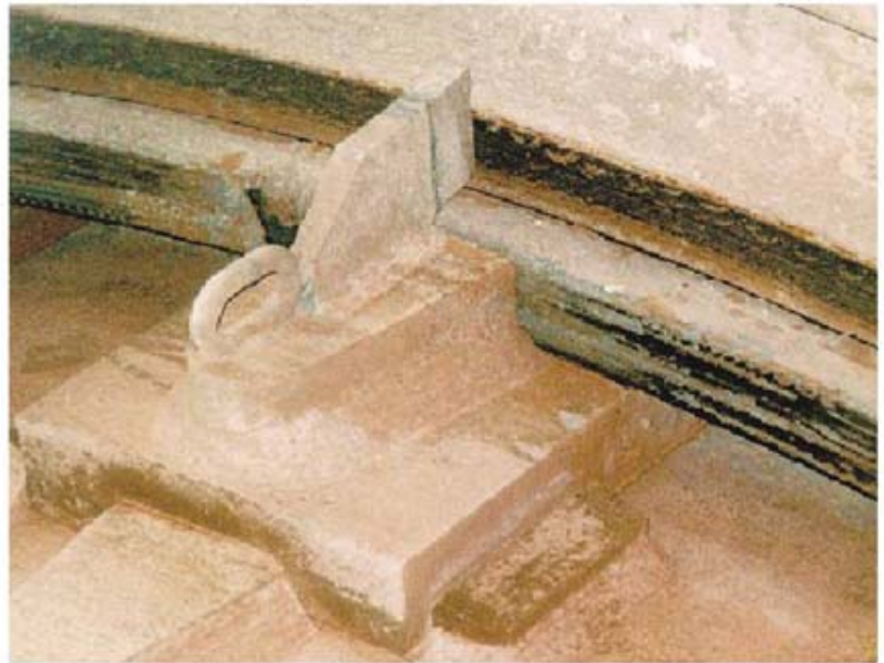
Wear and scuffing marks on surfaces of live rings and supporting blocks due to lack of lubricant
