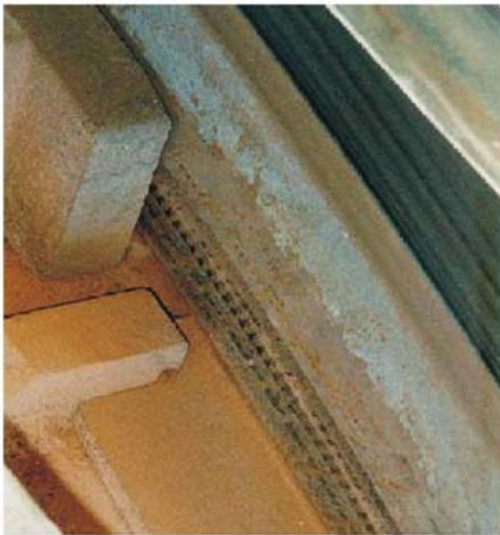
Wear and scuffing marks on surfaces of live rings and supporting blocks due to lack of lubricant
